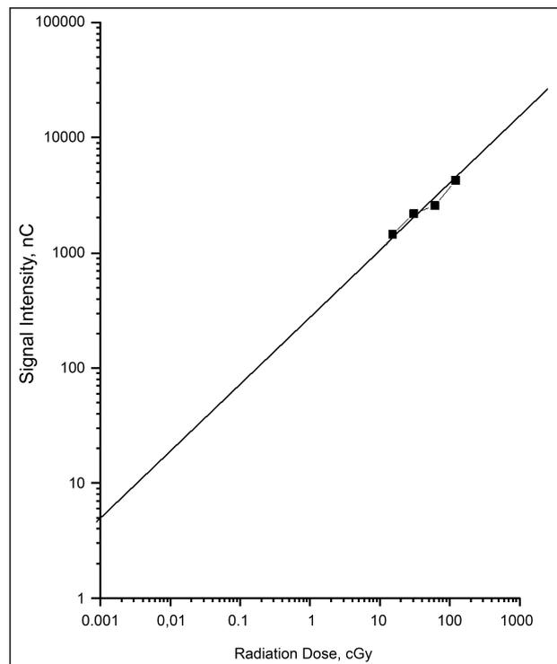
**Figure 1.** Calibration curve for measurement of radiation dose by thermoluminescent dosimeter.
