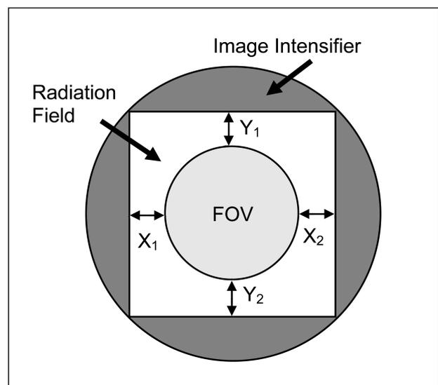
**Figure 3.** Schematic diagram of quality assurance test for matching x-ray field with the field of view (FOV) in fluoroscopy. The inner circle is the FOV and the outer rectangular area is the x-ray field. The error (excess of x-ray field over the FOV) on x-axis is  $X_1+X_2$  and that on y-axis is  $Y_1+Y_2$ .
