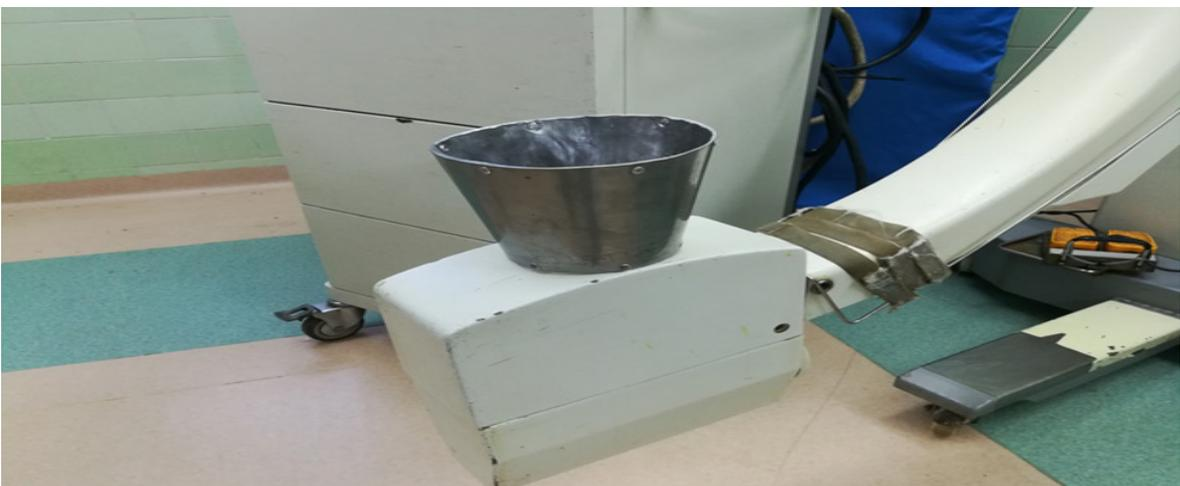
**Figure 3.** Fluoroscopy tube with designed lead connector.
