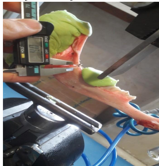
Figure 2: Load application to measure the fixation strength
