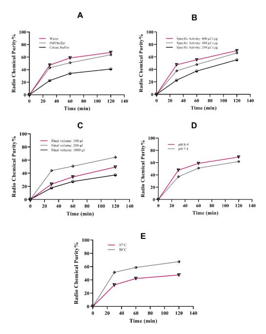
**Figure 2.** Influence of type of buffer (A), specific activity (B), final volume (C), pH (D), and temperature (E) on radiolabelling of His-tagged scFv with <sup>99m</sup>Tc-tricarbonyl. RCP of the radiolabeled scFv ( $n = 3 \pm SEM$ ) was evaluated at 0, 30, 60, and 120 min.
