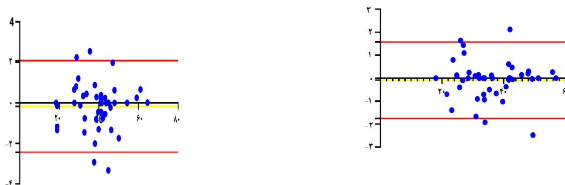
Figure 5: Bland-Altman plot to show the difference versus the mean of lordosis results on a) Microsoft Kinect, b) Flexible Ruler
