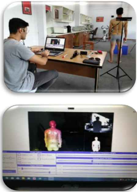
Figure 1: measure the spine using the Kinect Marusoft camera
