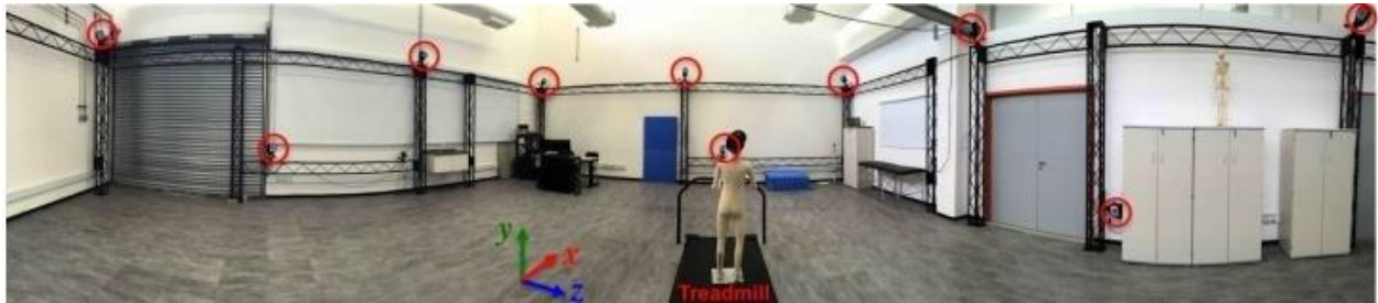
Figure 1. Overview of the Laboratory of Biomechanics and Motor Control. Expanded view of the Laboratory of Biomechanics and Motor Control (BMClab), showing 10 of the 12 motion-capture system cameras (marked with red circles), the instrumented treadmill, and the laboratory coordinate system
