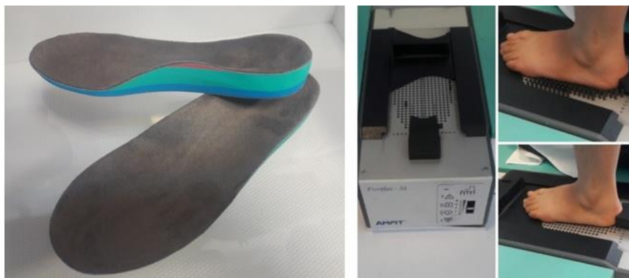
Figure 1. Right image: 3D scan, left image: Semi-rigid custom insoles with fabric cover
