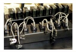
Figure 1. Eight-Channel Electromyography Noraxon Device.
