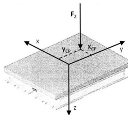
**Figure 2.** Determine the Center of Pressure Using Measured Forces and Moments.<sup>13</sup>
