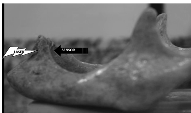
Figure 1. Laser Placed in the Apical Region at the End of the Dental Alveoli and the Sensor Positioned in Direct Contact With the Surface on the Bone Wall Opposite to the Radiated Wall.
