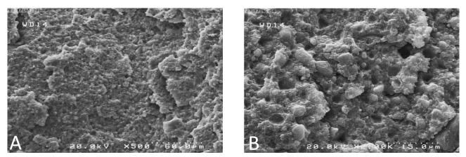
Figure 5 (A, B). Surface treated by Er:YAG laser with power of 5 W, 250 mJ (Original magnification x500, x2000)
