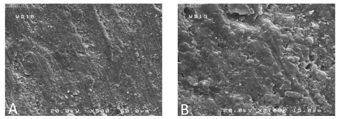
Figure 7 (A, B). Surface treatment by bur (Original magnification x500, x2000)
