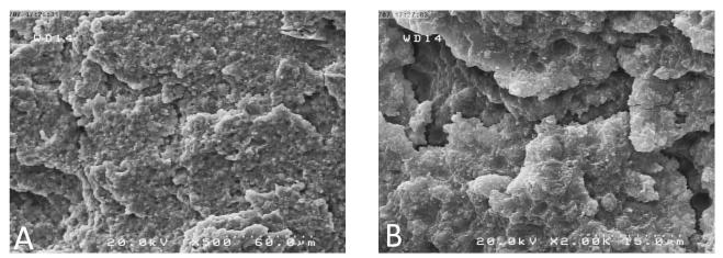
Figure 2 (A, B). Surface treated by Er:YAG laser with power of 2 W, 100 mJ (Original magnification x500, x2000)
