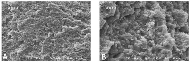
Figure 3 (A, B). Surface treated by Er:YAG laser with power of 3 W, 150 mJ (Original magnification x500, x2000)
