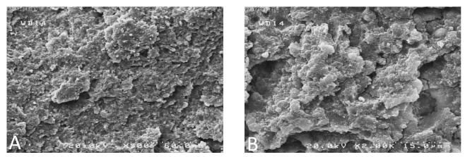
Figure 4 (A, B). Surface treated by Er:YAG laser with power of 4 W, 200 mJ (Original magnification x500, x2000)
