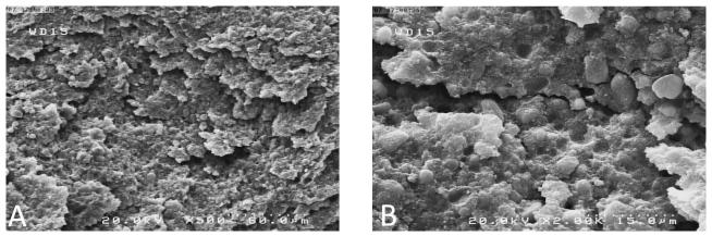
Figure 6 (A, B). Surface treated by Er:YAG laser with power of 6 W, 300 mJ (Original magnification x500, x2000)
