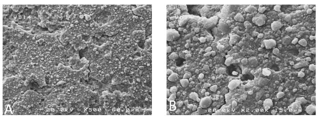
Figure 1 (A, B). Surface treated by Er:YAG laser with power of 1 W, 50 mJ (Original magnification x500, x2000)
