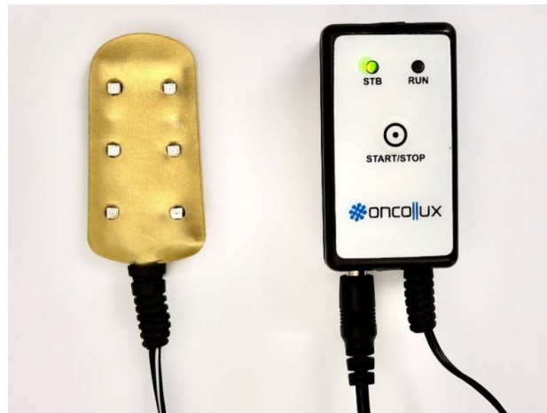
Figure 1. LED Plate Used for photobiomodulation in the Present Study (Odontollux®, Cosmedical, Brazil)
