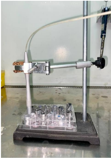
Figure 1. Low-Power Laser Irradiation in a Non-contact Mode
