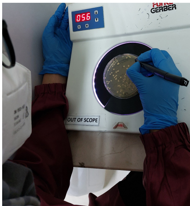
Figure 4. Colony Counting Using a Colony Counter
