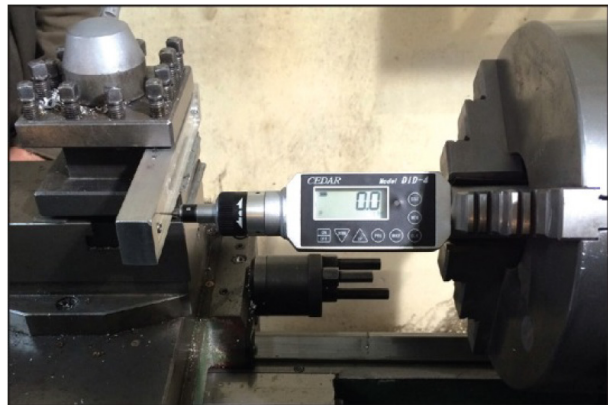
Figure 2. Torque Testing Setup (Milling Machine, Torque Tester, Custom-Made Screw Driver, Mini-screw and Polycarbonate Plate)
