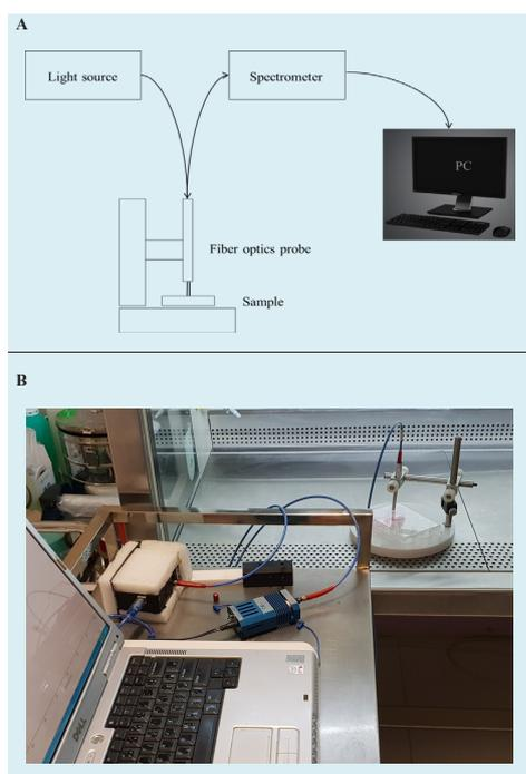
**Figure 2.** A) Laboratory layout of optical reflectance spectroscopy of cell samples and B) optical reflectance spectroscopy.
