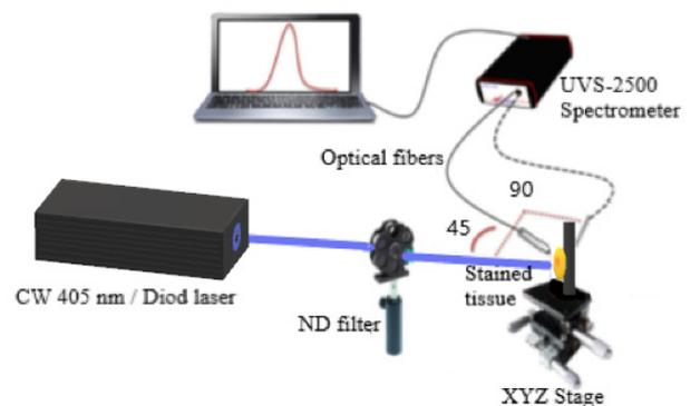
Figure 1. The Schematic of LIF Set-up for the NaFl-Stained Tissues.
