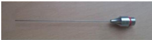
**Figure 10.** Cannula Used to Insert Optical Fiber Into Tissue.
