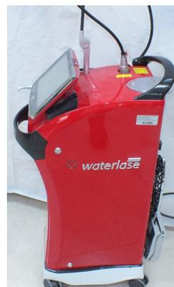
Figure 2. Er, Cr:YSGG Waterlase Laser Device.
