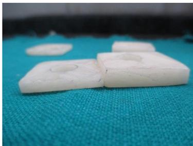
**Figure 3.** Spacer of 3 mm and 6 mm Thickness.
