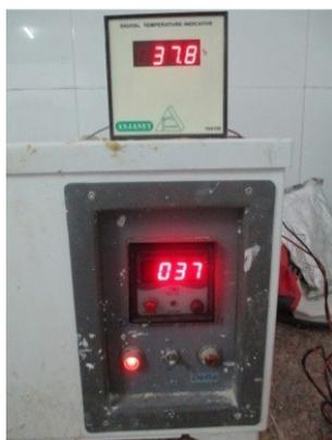
**Figure 10.** Digital Thermometer (connected with thermocouple) is kept over waterbath, showing intrapulpal temperature change.
