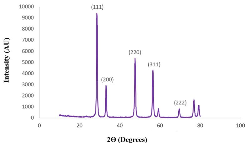
**Figure 1** XRD pattern of green synthesized CeNPs
