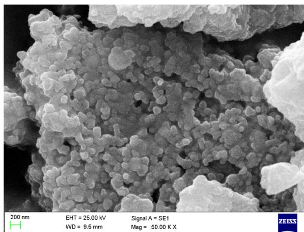
**Figure 2.** SEM imaging of synthesized CeNPs
