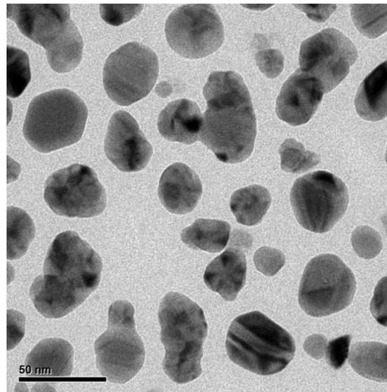
Figure 3. TEM imaging of synthesized CeNPs
