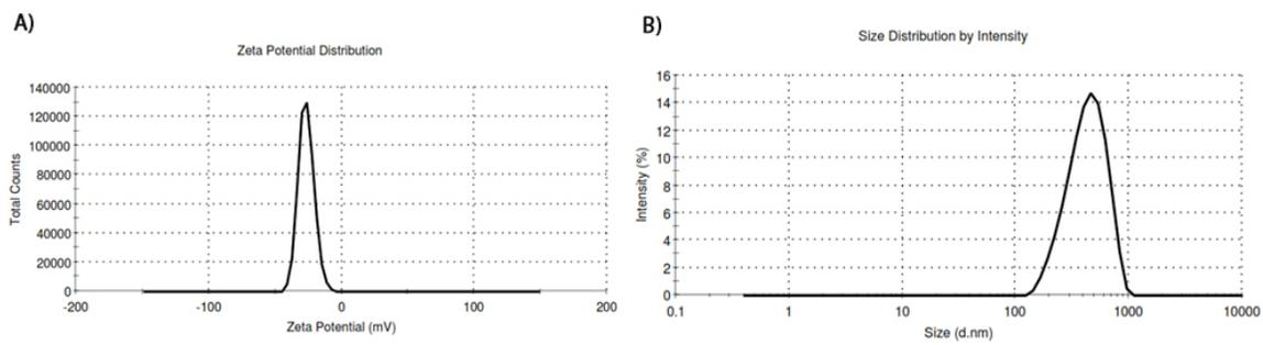
Figure 4. (A) Zeta potential of synthesized nanoparticles and (B) hydrodynamic radius of synthesized nanoparticles
