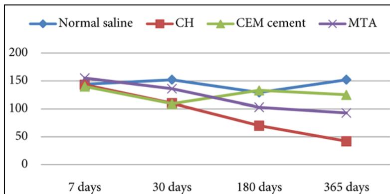
Figure 1. Flexural strength means (MPa) for each group
