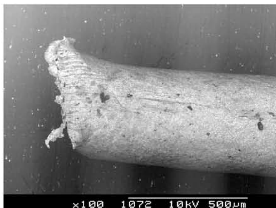
Fig1. Scanning electron micrograph of Gutta-Percha Cone cutting with scissors. There are two plane and convergent flange (original magnification \times 100 ).
