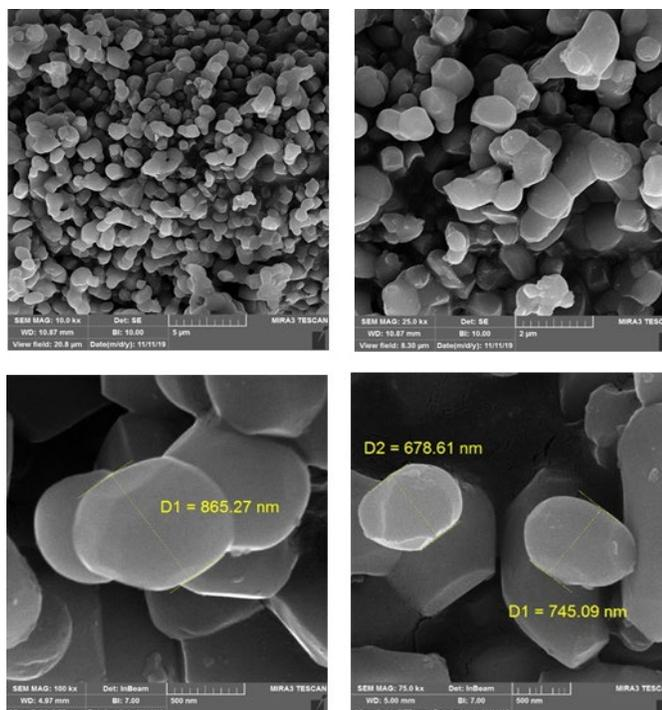
Figure 1. SEM micrographs of ceramic microparticles; exhibiting acceptable size and proper smooth surfaces; appropriate for drug delivery
