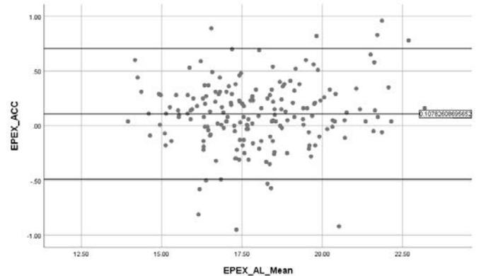
Figure 5. The Bland-Altman plot for the agreement of E-Pex Pro and actual length measurement
