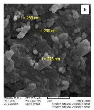
**Figure 1.** SEM images of non-conjugated MWCNTs (A), and conjugated CNTs with drug (B).
