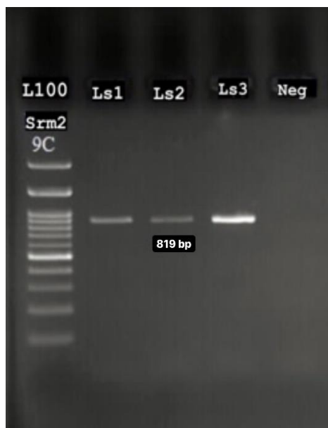
Figure 2. HBV pres/s amplification products electrophoresed on a 1.5% agarose gel L: Ladder 100-1000 bp, Ls: Left area of the pre s/s region, N: Negative control.
