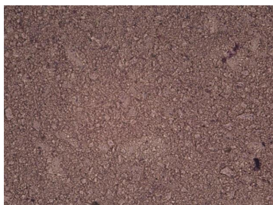
Figure 1: Filler distribution of Trimed composite using the Lapping method
