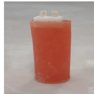
Figure 1: Zirconia cube mounted in an acrylic block with 4 cylinders made with resin cement
