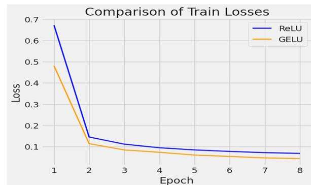
Figure 10: Performance comparison of train losses using different activation functions in dense layer of the proposed model.
