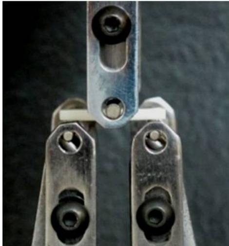
**Figure 1- Bar-shaped specimen placed on the two jigs. Load was applied from the top by the blade for TPFS testing**
