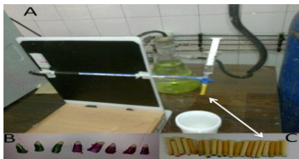
Figure 2- (A) Fluid filtration apparatus (B) External surfaces of samples were covered with two layers of nail varnish and one layer of cyanoacrylate glue from the coronal edge to 2.0 mm short of the apex. (C) Teeth are ready for placement in the apparatus.
