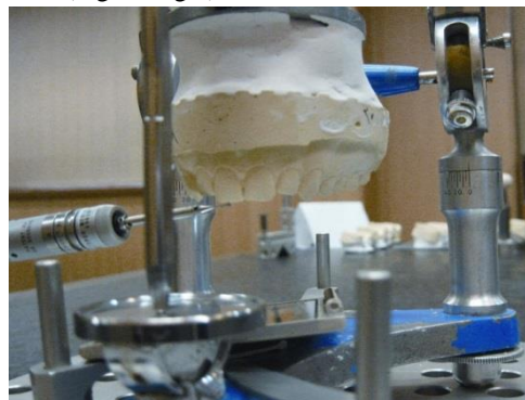
Figure 1- Contact of probe of C.M.M to the spots marking the mesial and the middle point on incisors
