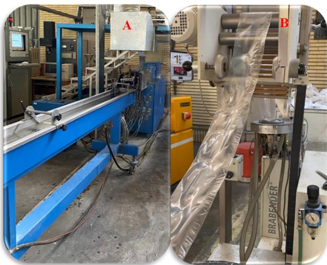
Figure 1. The film processing. A, extruder machine; b, film layers
