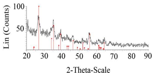
**Figure 3.** X-ray diffraction pattern of the prepared nanostructures, indicating characteristic peaks of akaganeite crystals. (■)  $\beta$ -FeOOH JCPDS Card No. 75-1549
