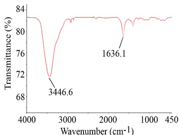
**Figure 4.** Fourier transform infrared spectrum of the bio-assisted synthesized FeOOH nanoellipsoids, indicating virgin nanostructures with no impurities
