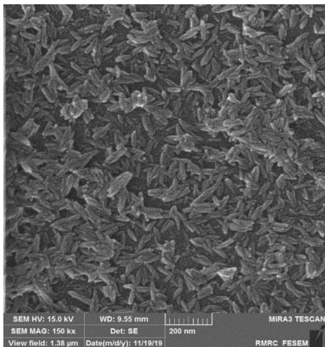
**Figure 1.** A field-emission scanning electron microscopy micrograph of the bio-assisted synthesized FeOOH nanoellipsoids
