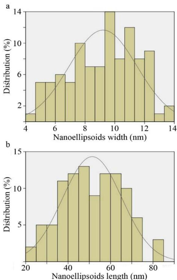
**Figure 2.** Nanoellipsoids width (a) and length (b) distributions. Measurements were carried out on field-emission scanning electron microscopy micrographs
