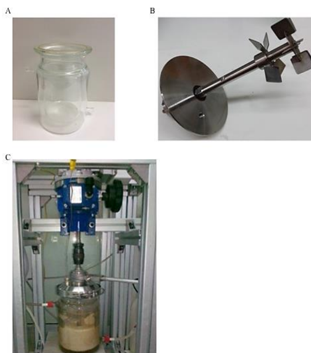
Figure 1. The vessel, mixing system and bioreactor. A) The vessel was built using Pyrex and equipped with an external jacket that allowed the circulation of service fluid necessary to maintain the entire apparatus at a constant temperature. B) The stainless steel impeller with two various types of turbines: a blade turbine to reach an axial flow and a Rushton turbine to reach a radial flow. C) The complete equipment was used for the lab-scale experiments.
