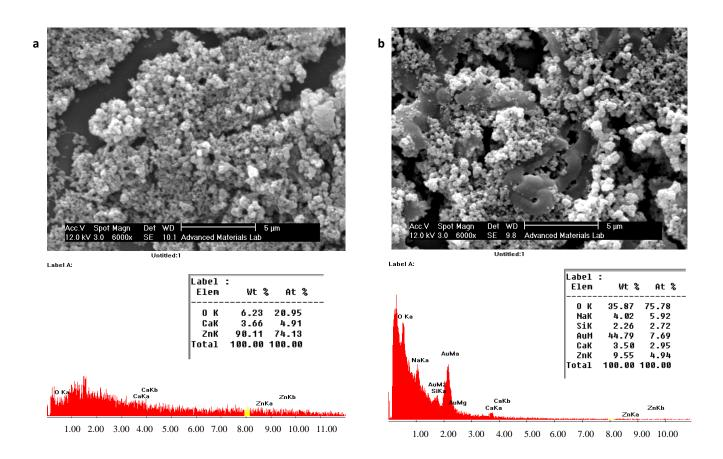
**Figure 5**. The SEM image and EDXS of BH4 strain immobilized on chitosan-TPP gel beads. a) Chitosan gel treated with zinc oxide (1 mg  $l^{-1}$ ); b) Chitosan gel without nanoparticles. Based on the elemental dispersion analysis (using EDXS device attached to SEM), where zinc oxide nanoparticles are further cross-linked, the particles are further coherent and better immobilized.
