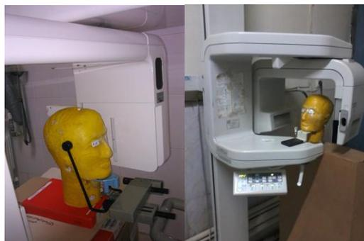
**Figure 2.** Phantom placement in analogue (left) and digital (right) devices
