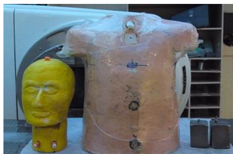
Figure 2. Anthropomorphic phantom with the depth TLD applicators.
