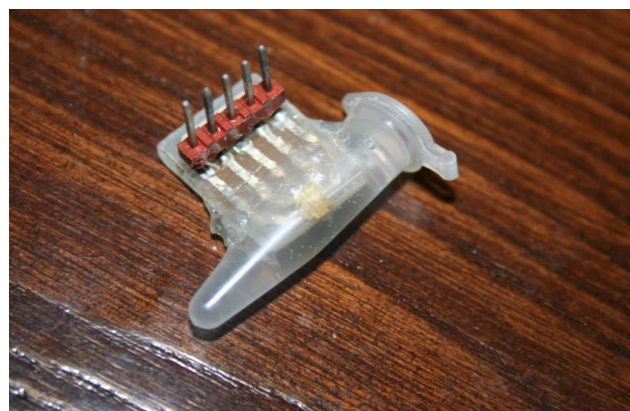
Figure 3. Microcantilever was stabilized in a plastic micro tube and after immobilization of enzyme, subsequent tests were done in contact with immobilized MAO on the microcantilever.
