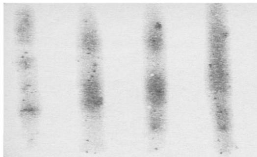
Fig (6): The radiographic image of compacted cellulose with pasted barium sulfate strips that both have the same thickness of 300 $\mu$ . The atomic number and density difference between two materials is close to that between muscle and fat tissues.
