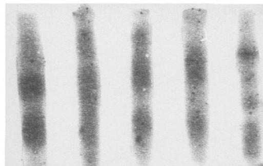
Fig (7): The radiographic image of sheet phantom that the density difference between strips and sheet is similar to that between bone and muscle tissues.
