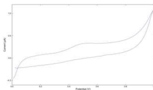
**Figure 2.** Cyclic voltammogram of the RGO-AuNPs nanocomposite in 100 mM acetate buffer, pH 4.6 at 25 °C. Scan rate: 100  $\text{mVs}^{-1}$ . Scan range: 0.0–1.0 V.
