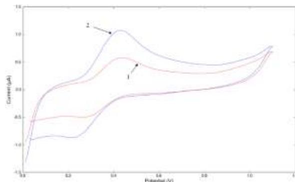
**Figure 4.** Cyclic voltammograms of the laccase immobilized using the RGO-AuNPs/PNR nanocomposite in buffer (1) and in presence of 10 mM syringaldazine (2) in 100 mM acetate buffer, pH 4.6 at 25 °C. Scan rate: 100 mVs<sup>-1</sup>. Scan range: 0.0–1.0 V
