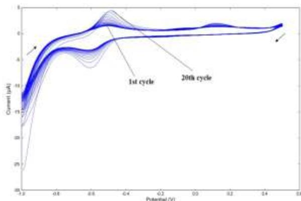
**Figure 3.** Cyclic voltammogram of the electro-synthesis of PNR on AuNPs/RGO in 100 mM potassium phosphate buffer, pH 5.5 at 25 °C. Scan rate: 100 mVs<sup>-1</sup>. Scan range: -1.0–0.6 V
