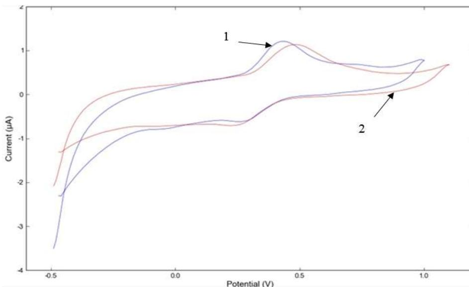
**Figure 6** Cyclic voltammograms of RGO-AuNPs/PNR/laccase modified electrode after 1 day and 10 days of starvation in the 100 mM acetate buffer at pH 4.6 and 25 °C. Scan rate: 100 mVs<sup>-1</sup>. Scan range: -0.5–1.0 V.
