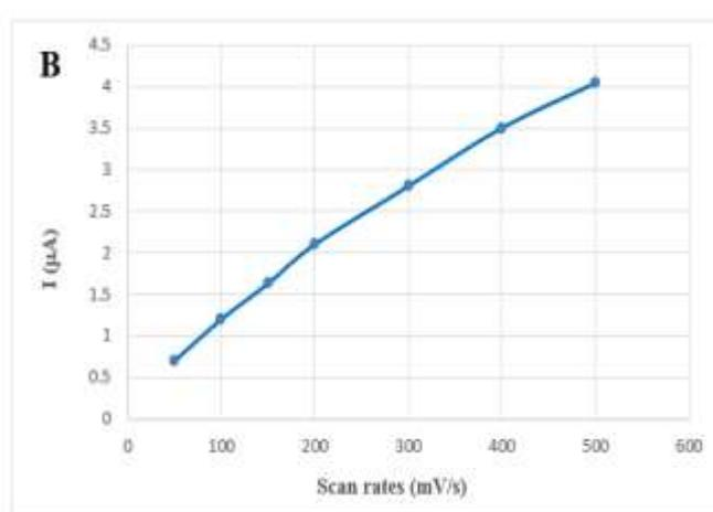
**Figure 5.** (A) Cyclic voltammograms of the laccase immobilized onto RGO/AuNPs/PNR nanocomposite at a scan rate of 50,100,150,200,300,400 and 500 mVs<sup>-1</sup> in 100 mM acetate buffer, pH 4.6 at 25 °C. Scan range: 0.0–1.0 V. (B) Relation between the cathodic current peaks and different scan rates of presented biocathode
