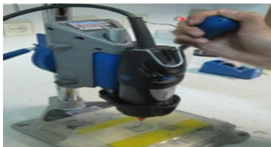
Figure 1. Production of a hole on FTO glass by using of drill press
