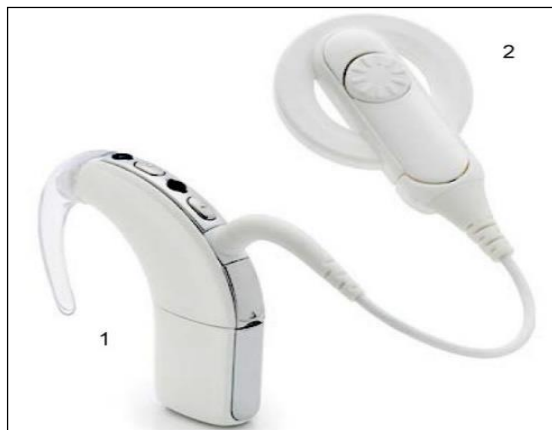
Figure 1. External component of a cochlear implant: (1) behind the ear sound processor; (2) antenna with a magnet (Taken from open access article) (5).
