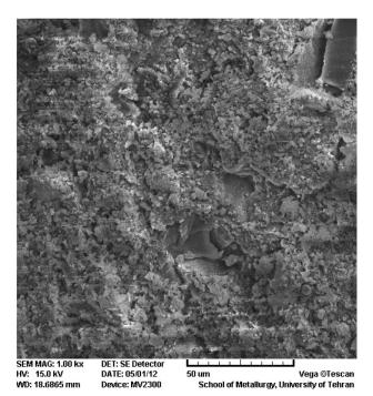
**Figure 6.** Surface treated by Er:YAG laser with output power of 7 W, 350 mJ (Original magnification ×1000, bar=50µm)
