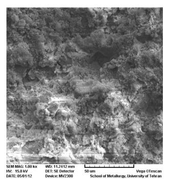
**Figure 5.** Surface treated by Er:YAG laser with output power of 6 W, 300 mJ (Original magnification ×1000, bar=50µm)
