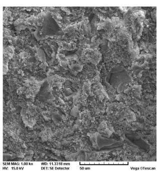
DATE: 05/01/12 Device: MV2300 School of Metallurgy, University of Tehran Figure 3. Surface treated by Er: YAG laser with output power of 4 W, 200 mJ (Original magnification ×1000, bar=50μm)
