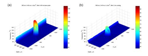
**Figure 2.** Calculated Temperature Distribution in the Tissue and Vessel According to the Depth and Transverse Coordinate. A vessel with a diameter of 300 mcm was assumed located at a depth of 500 mcm for PDL fluence of 4 J/cm<sup>2</sup> (a- maximum heating at the end of PDL pulse, b- 3 msec after the end of PDL pulse).
