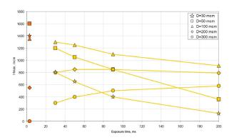
Figure 3. Calculated maximum depth, at which the vessel could be heated entirely up to  $75^{\circ}$ C using PDL at 585 nm (orange dots) and CVL at 578 nm(yellow dots).
