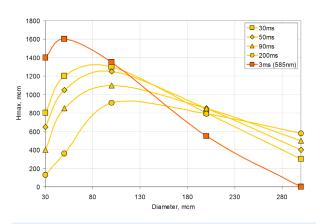
**Figure 4.** Calculated maximum depth, at which the vessels of different diameters could be heated entirely up to the temperatures higher than 75°C using PDL at 585 nm(orange line) and CVL at 578 nm(yellow line) with different exposure time.
