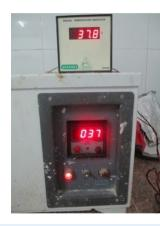
**Figure 10.** Digital Thermometer (connected with thermocouple) is kept over waterbath, showing intrapulpal temperature change.
