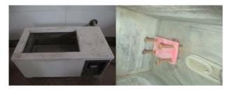
Figure 7. Waterbath Equipment for Controlled Water Temperature.
