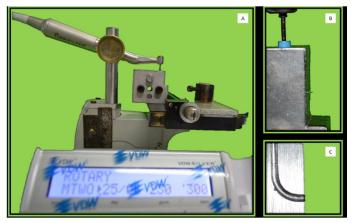
*Figure 1.* Supporting device for the artificial canal and the cyclic fatigue test. *A*) Counter-angle x file ratio x stainless steel apparatus used in the cyclic fatigue test; *B*) File tip out of the canal; *C*) Characteristics of the artificial canal geometry.
