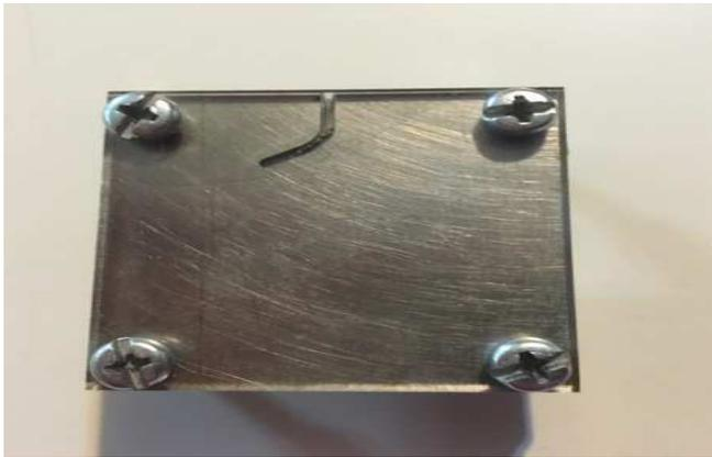
Figure 1. Artificial stainless steel canal
