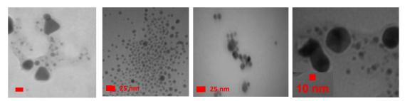
*Figure 2.* TEM images of the synthesized AgNPs. *A*) C<sub>12</sub> Pyridinium-coated; *B*) C<sub>18</sub> Pyridinium-coated; *C*) C<sub>12</sub> Imidazolium-coated; *D*) C<sub>18</sub> Imidazolium-coated
